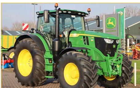
John Deere 6R215, nieuw, Autopower 40 km/u, banden 710/60R42 en 600/65R28, Autotrac, fronthef, LED lampen
